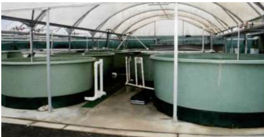
Figure 12 - Queenscliff mussel hatchery 5t settlement tanks (DEPI)
